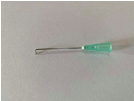
21 gauge needle with tip removed and end bent to 90 degrees
